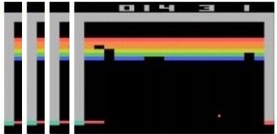
Current state s_t : 84x84x4 stack of last 4 frames (after RGB->grayscale conversion, downsampling, and cropping)
